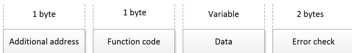
Fig.3 general MODBUS frame
